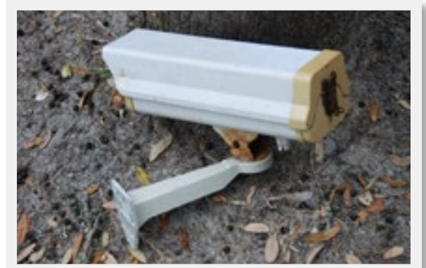
This camera case was up for 7 months and failed.
